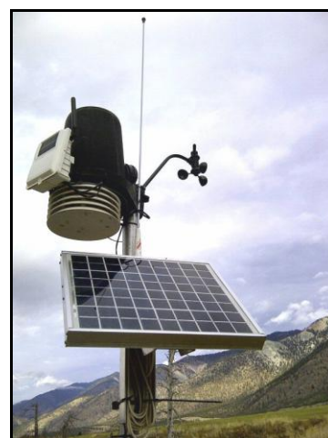
Instrument panel of Davis Pro 2 weather station at Half Way Ranch and Diamond- S Ranch with solar panel and wind gauge.
